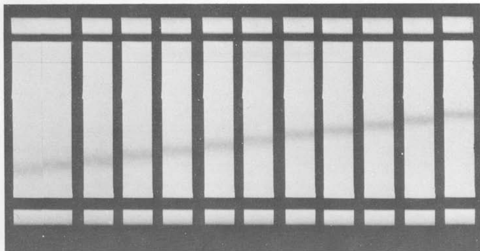
FIGURE 3. Band sedimentation pattern of a mixture of equal amounts of TNV (strain from Dr. M. K. Corbett) and of the citrus isolate of TNV. Sedimentation velocity, 20,410 rpm.
