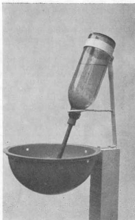
Fig. 2. Refilling device used for yellow pan aphid traps.
